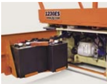
All-steel swing-out battery doors with heavy-duty hinges.
